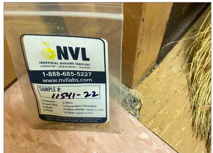
Photo #4: Sample 11541-22: Various colored 9'x9' vinyl composite tile & various colored 12'x12' vinyl composite tile on ACM black mastic (3% Chrysotile) on concrete Location: Throughout 1 st Floor Quantity: 24,000 SF
