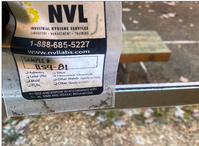
Photo #5: Sample 11541-81: ACM Black window caulking (2-3% Chrysotile) on metal frame windows 7'x7'
