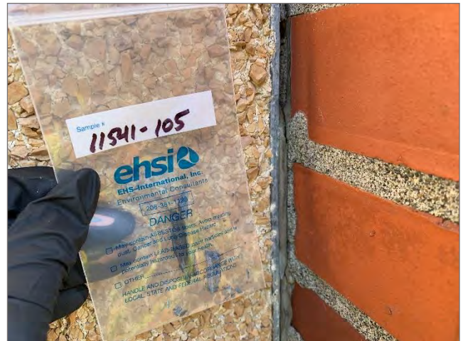
Photo #6: Sample 11541-105: ACM Gray caulking (2% Chrysotile) joining brick/marblecrete
