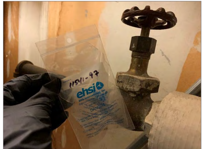
Photo #14: Sample 11541-97: ACM Residual TSI (<1-20% Chrysotile, 15% Amosite) on pipe Location: Throughout Quantity: 5 SF
