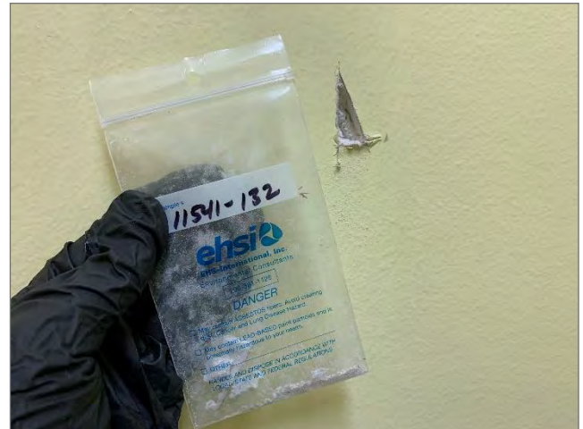
Photo #10: Sample 11541-132: ACM White jc (2-3% Chrysotile) on GWB * <1% when composited as part of GWB system Location: Throughout First Floor Quantity: 4,000 SF
