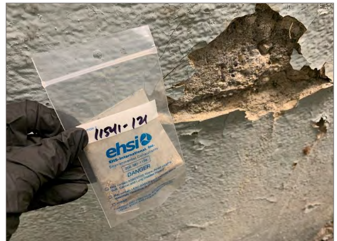
Photo #8: Sample 11541-121: White skim coat (2% Chrysotile) on concrete walls
