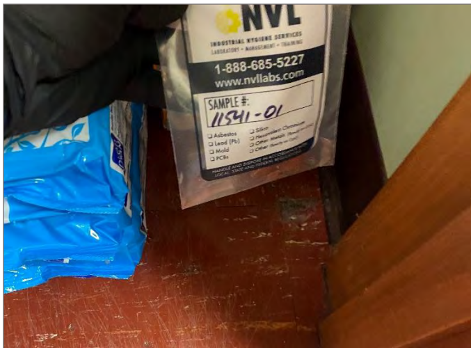
Photo #1: Sample 11541-01: ACM Red 9'x9' vinyl tile (6% Chrysotile) on black mastic (on concrete) Location: Throughout Office Quantity: 3,000 SF
