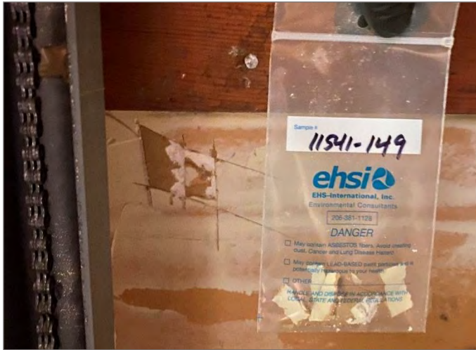
Photo #13: Sample 11541-149: ACM White jc (2% Chrysotile) on GWB * <1\% when composited as part of GWB system Location: Throughout Second Floor Quantity: 5,600 SF
