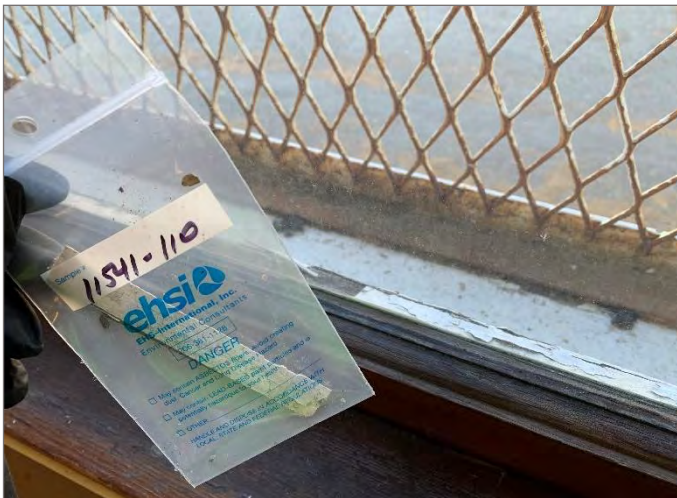
Photo #15: Sample 11541-146: ACM Gray glazing (3% Chrysotile) on wood frame window Location: P-1 / P-2 Quantity: 300 SF
