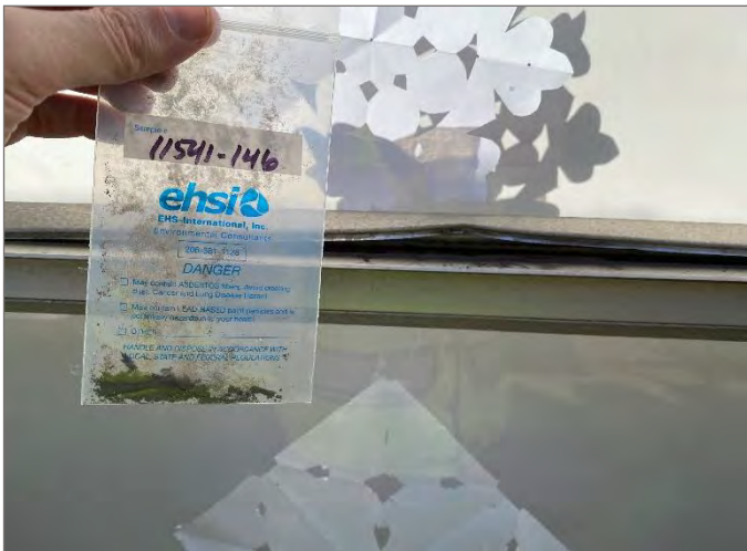
Photo #11: Sample 11541-146: ACM Gray caulking (4% Chrysotile) on metal frame window 5'x7' Location: Throughout Exterior Quantity: 540 SF / 30 EA
