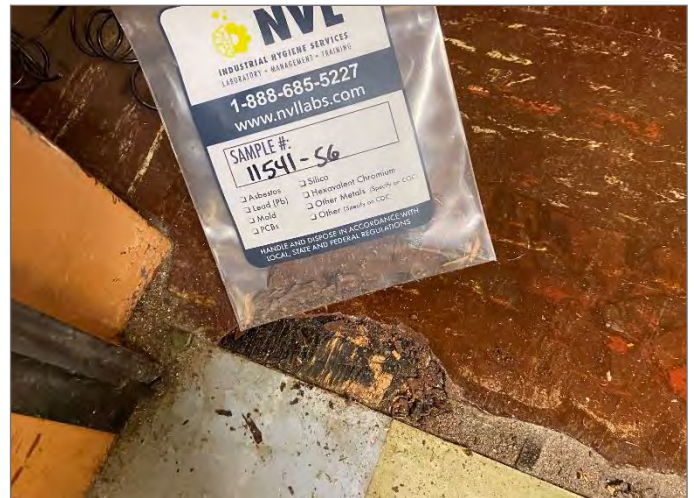
Photo #12: Sample 11541-56: ACM dark brown 9'x9' vinyl tile (3-4% Chrysotile) on black mastic (on wood) Location: Throughout Second Floor Quantity: 260 SF
