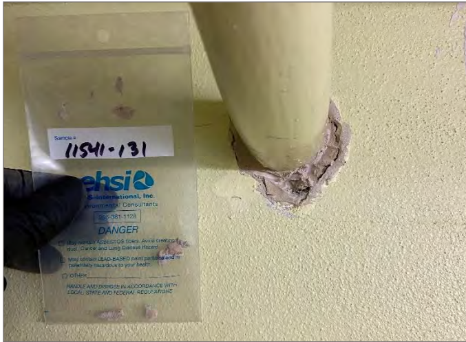
Photo #9: Sample 11541-131: ACM Beige firestop (2% Chrysotile) on GWB Location: Stock Room Quantity: <2 SF
