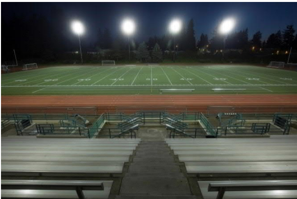
Direct glare from unshielded floodlights (Edmonds-Woodway HS), Reflected glare from synthetic turf surface.
