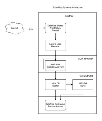
The diagram provides a high-level view of our system architecture. Detailed schematics of all system and network architecture are audited annually by a QSA (Qualified Security Assessor) as part of our annual, Level One PCI DSS audit. Some of the network diagrams are proprietary to our hosting provider who is SAS 70 Certified and considered to be the gold standard in PCI DSS Hosting solutions.
