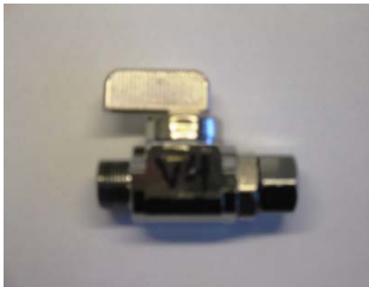
Figure 7. Stagnation testing in quadruplicate of a typical brass shutoff valve. (a) Lead concentration in tap water as a function of cumulative exposure and (b) enlarged view of brass shutoff valve.
