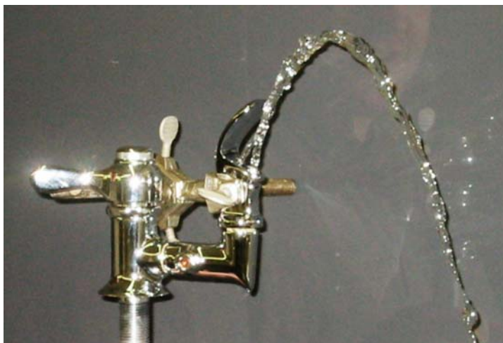
Figure 6. Lead concentration in tap water as a function of cumulative exposure of bubbler heads to tap water during (a) flow-through testing (Type A and Type B bubbler heads) and (b) stagnation testing (Type A bubbler head tested in quadruplicate). (c) Bubbler head with valve held opened during flow-through testing.
