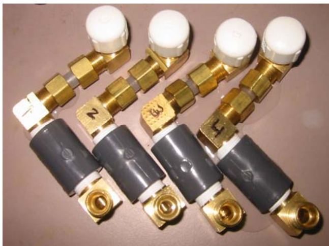
Figure 9. Stagnation testing in quadruplicate of three brass elbows linked together. (a) Lead concentration as a function of cumulative exposure to tap water and (b) specimens prepared for testing.
