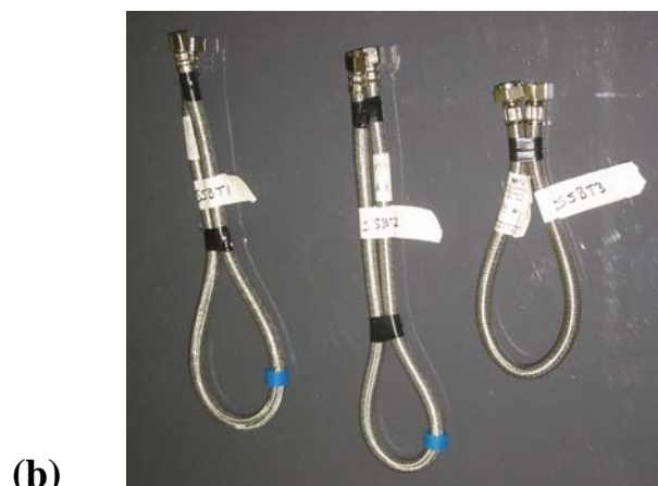
Figure 8. Stagnation testing in triplicate of a flexible connector with brass ferrules at both ends. (a) Pb concentration in tap water as a function of cumulative exposure time, (b) specimens prepared for testing, and (c) enlarged view of brass ferrule at one end of flexible connector.
