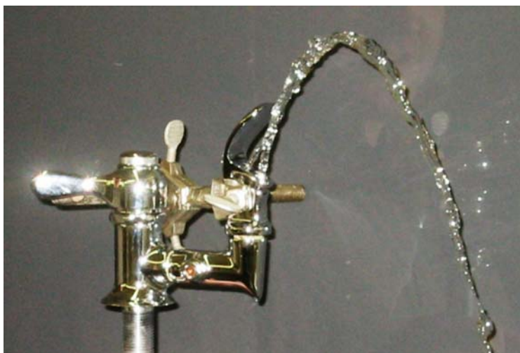
Figure 6. Pb concentration in tap water as a function of cumulative exposure of bubbler heads to tap water during (a) flow-through testing and (b) stagnation testing. (c) Bubbler head with valve held opened during flow-through testing.
