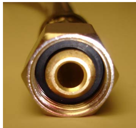
Figure 8. Stagnation testing in triplicate of a flexible connector with brass ferrules at both ends. (a) Pb concentration in tap water as a function of cumulative exposure time, (b) specimens prepared for testing, and (c) enlarged view of brass ferrule at one end of flexible connector.
