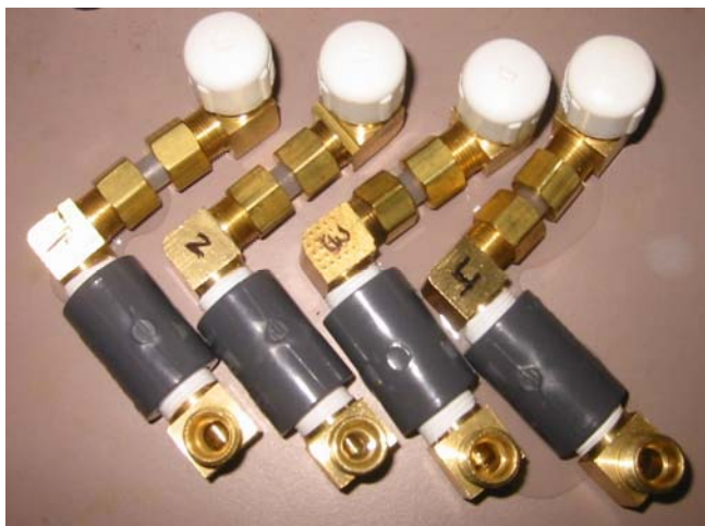
Figure 9. Stagnation testing in quadruplicate of three brass elbows linked together (a) Pb concentration in tap water as a function of cumulative exposure to tap water and (b) specimens prepared for testing.
